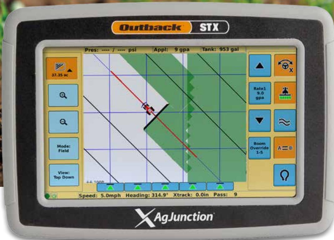
The Outback STX™ Guidance System is the culmination of combining full RTK capability along with rate and section control in an autosteer ready, value based terminal. The Outback STX incorporates some of the industry's best innovations in a system priced below competitive terminals in this segment of the market.
